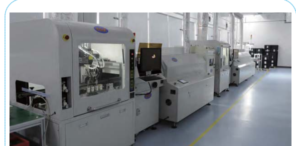
Note: The automatic spraying process of conformal coatings
